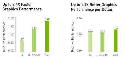
1 Comparison of NVIDIA A40 virtual workstation to NVIDIA T4, RTX 6000 and RTX 8000 virtual workstations, 1 user per board, running on a server configured with 646B RAM per user. SPECviewperf results tested on a server with 2x Xeon Gold 6154.3.0GHz (3.7GHz Turbo), VMware vSphere 7.0 U2, host/guest driver 670.63. NUDIA RTX vwS 13 I SPECviewperf 2020, 4K Geomean
