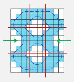
**Mango** – This character classifier uses 8x5 grid matrix matching to identify features classified with a k-NN algorithm. It also contains a decision tree-based "super classifier" that takes as input the output from the other classifiers to produce an even more reliable result.
