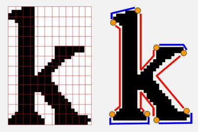
**FireWorx** – This classifier has two components. The first component is a matrix matcher CV algorithm that partitions characters into a 12x12 grid (144 binary values). These grids are fed into a fuzzy AI decision-tree classifier that performs bit-by-bit comparisons of interesting leaves. The second component uses a chain code histogram to identify the contour steps. These are then fed into a neural network classifier.
