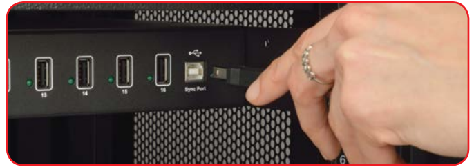
The USB uplink port connects to a computer for device syncing.
