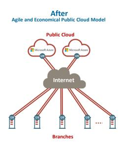
The 128T Session Smart Networking solution provides efficient, secure, resilient internet connectivity for branch offices scattered across the United States. The 128 Technology solution manages and controls individual traffic flows at the edge, based on policy, helping the firm ensure superior user experiences for cloud applications. Redundant uplinks and fast failover capabilities ensure continuous availability in the event of ISP outages or link failures.
