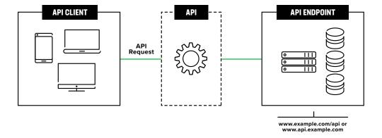
Figure 1: Web APIs connect to an endpoint: the location of the web server and supporting databases
