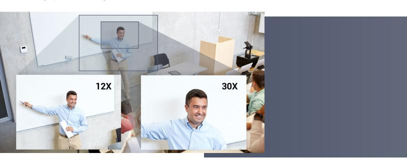
Digital zoom on the other hand, is your camera's software at work with digital processing to alter the image. As others have stated, digital zoom is an "invention of digital video cameras" and it enlarges the target image which can blur or degrade the quality of the video. While this type of zoom has its uses, to produce high quality video with live streams, optical zoom is the only true measure to review.
