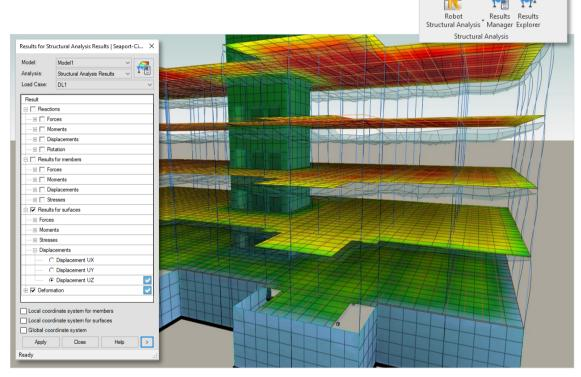
Structural analysis visualization tools are now integrated into Revit
