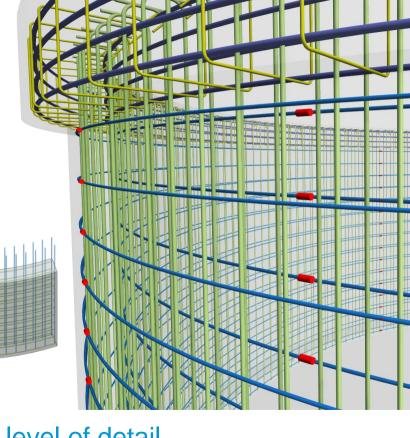
Model arc-shaped reinforcement at a higher level of detail
