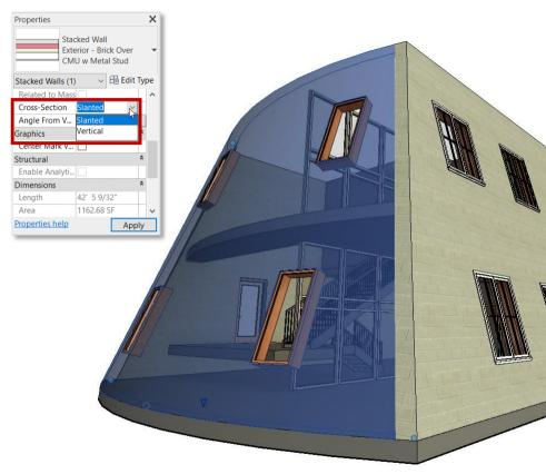
Easily model slanted architectural, structural, and curtain walls.
