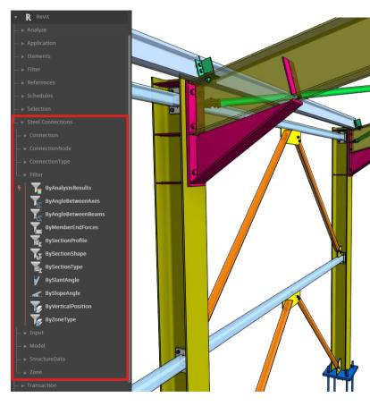
Dynamo nodes for steel connections are now installed with Revit
