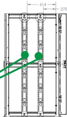
Horizontal cable channels allow for front-to-rear cable management inside the sidecar and prevent sagging of large bundles of cable.
