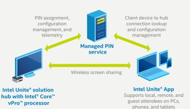
The on-premise option features an Intel Unite® solution PC hub,
