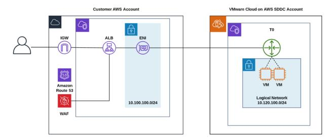
The reference architecture illustrates a VMware virtual machine web server workload that is running in VMC. Our solution uses Amazon native services to provide a solution for DNS name resolution, web traffic filtering, DDoS protection and load balancing.
